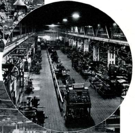
One of the bays at the Works of Messrs. Alfred Herbert, Coventry, that are lighted by 500w. Sieray-Dual Lamps.
