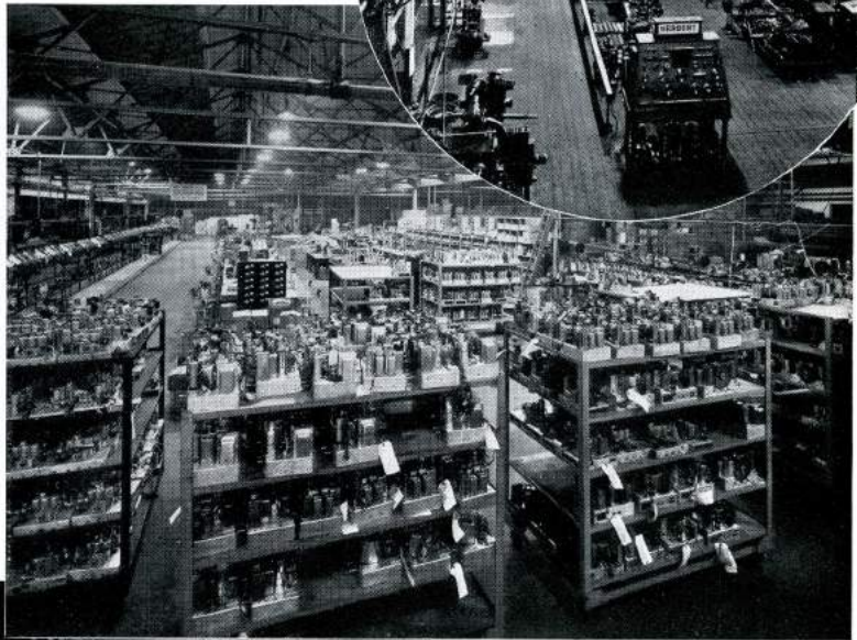
A Section of the Factory of Messrs. Philco Radio & Television Corporation of Great Britain Ltd., Perivale, which is lighted with 150w., 250w. and 400w. Sieray 'H' type Lamps.
