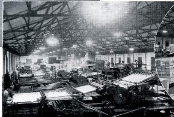
Printing Works illuminated by 400w. Sieray 'W' type Lamps.
